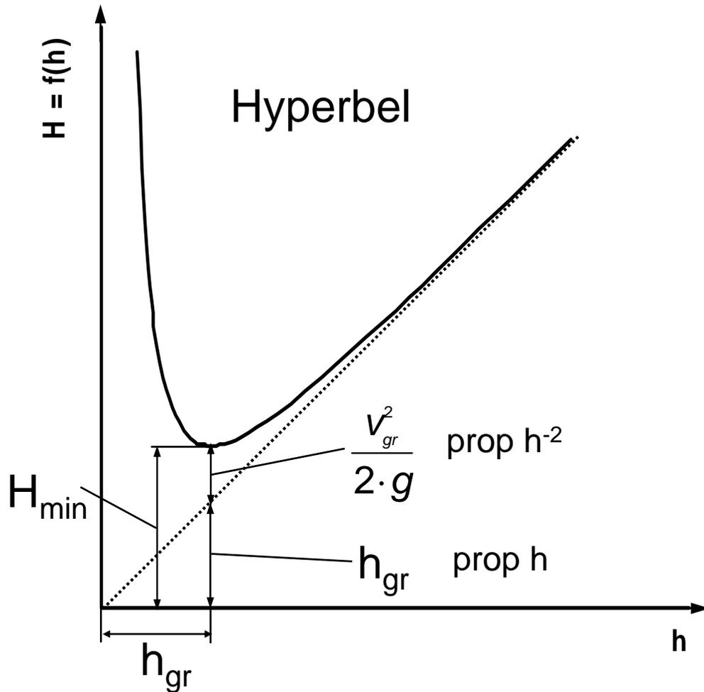
$$\min H = \frac{3}{2} h_{gr} = h_{gr} + \frac{v_{gr}^2}{2g}$$
