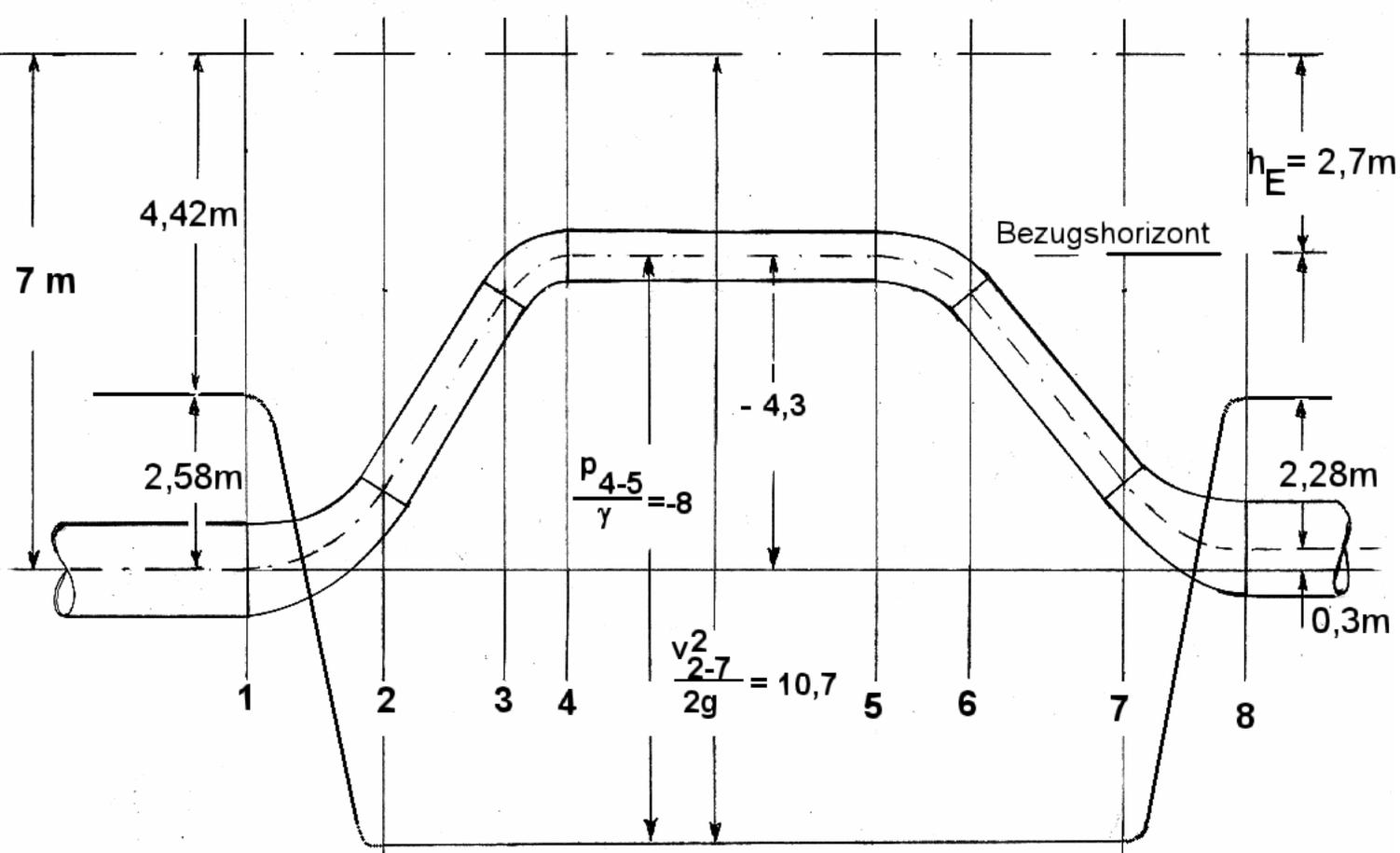
$$v_1 = \frac{Q}{A_1} = v_8 = \frac{Q}{A_8} = \frac{1,826}{0,196} = 9,316 \text{ m/s} \quad h_E = 2,7 = -4,3 + \frac{p_1}{\gamma} + 4,42 \rightarrow \frac{p_1}{\gamma} = 2,58 \text{ m}$$
