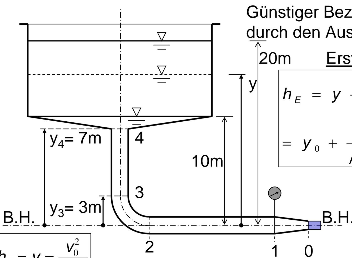
$$h_E = y = \frac{v_0^2}{2 \cdot g} \quad (\text{Toricelli})$$
